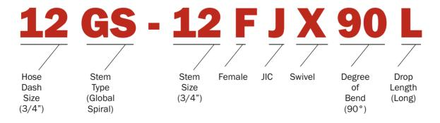
In the following example, the Gates description 12GS-12FJX90L identifies a GlobalSpiral Female JIC Swivel 90° Bend Long Drop coupling for -12 (3/4") hose size and -12 (3/4") stem size.
